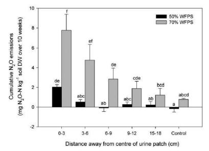
**Fig. 4.** Cumulative nitrous oxide emissions following sheep urine application to a Eutric Cambisol, maintained at either 50% or 70% water-filled pore space (WFPS) and sampled at increasing distances away from direct area of urine application. Bars represent means  $\pm$  SEM (n = 4) and different letters indicate significant differences (Fisher's LSD, p < 0.05).
